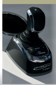
Instead of changing your heading via the CANtrak display, you can easily change your heading by tapping the joystick to get 1 degree or 10 degree changes in heading.
