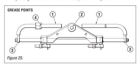
**1.** Remove support rod completely; clean engine steering/tilt tube. and regrease with a good quality marine grease. Complete on both sides of cylinder.
