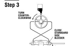
• Hold the cylinder body to prevent the rod from moving and turn the wheel counter-clockwise until a steady stream of air free oil flows from the bleeder nipple.
