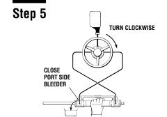
Hold the cylinder body to prevent the rod from moving a turn the wheel clockwise until a steady stream of air free oil flows from the bleeder nipple.
