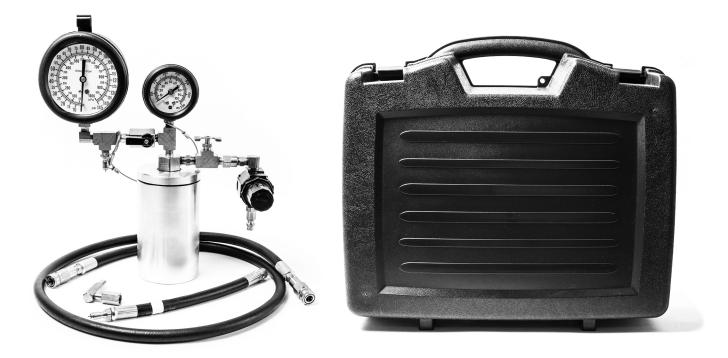
Step 1: Connect engine to hose or water source and run engine until it has reached operating temperature. <u>NOTE: For optimal performance, do not</u> attempt to clean a cold engine. Locate the Schrader valve and connect the fuel injection cleaner with the appropriate adaptor. Valve can be found either on the fuel rail or the VST Tank.
