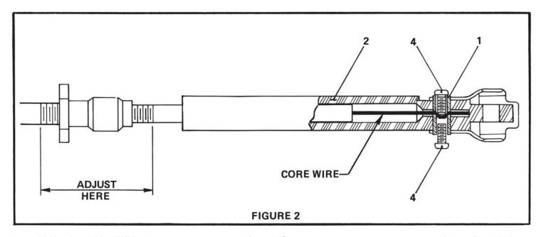
4. Holding assembly in place, thread one Clamp Screw (item 4) into Insert until it touches core wire, then add one more full turn. This kinks the core wire and helps prevent wire from pulling free. Thread second Clamp Screw (item 4) into opposite end of Insert until it touches core wire, then add one more full turn. DO NOT OVERTIGHTEN SCREWS. EXCESSIVE TORQUE MAY BREAK CORE WIRE.
