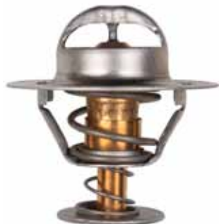
23-3604 THERMOSTAT Temperature Rating: 140° Replaces: Westerbeke 46097 Fits: 8.0 BEG(60Hz)/6.4 BEG(50Hz), 10.0 BEG(60Hz)/8.0 BEG(50Hz), 12.5 BEG(60Hz)/10.0 BEG(50Hz), 15.0 BEG(60Hz)/12.0 BEG(50Hz)
