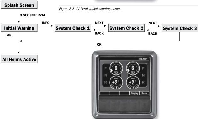
Figure 3-9. All Helms Active screen (normal steering mode).
