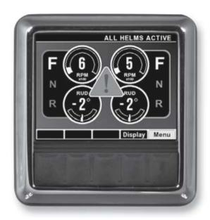
Figure 6-5. Run screen with system warning.
