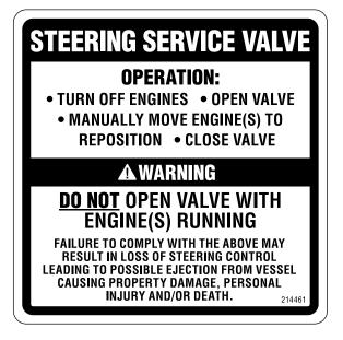
Figure 1-4. Steering service valve label.
