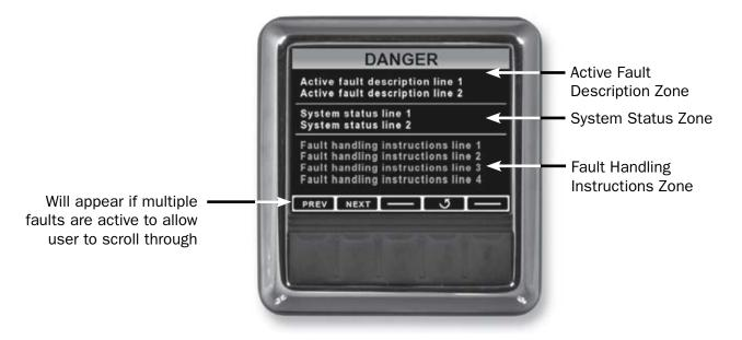
Figure 6-1. Danger fault screen layout.
