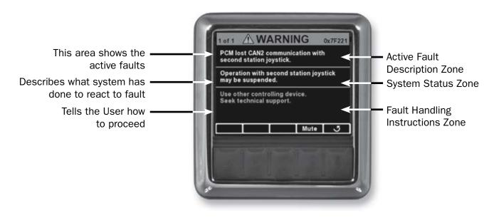
Figure 6-6. Sample warning fault.
