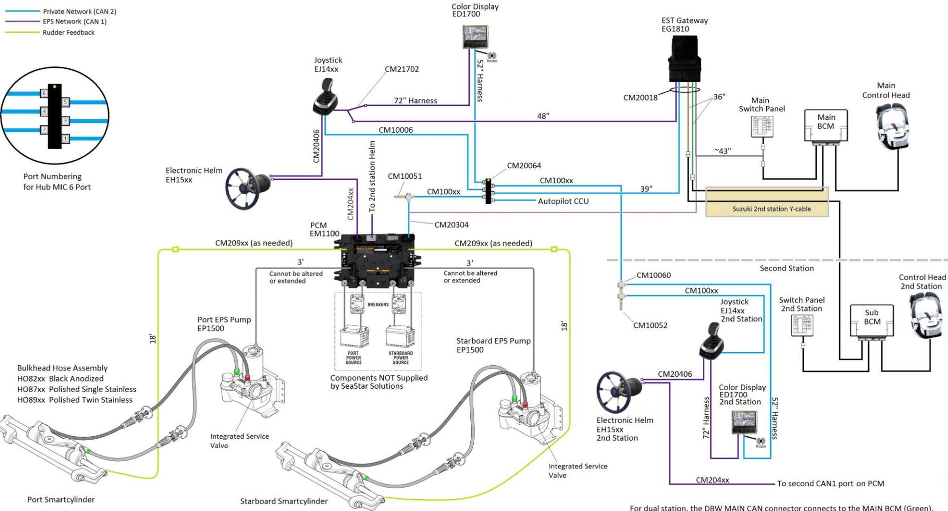
For dual station, the DBW MAIN CAN connector connects to the MAIN BCM (Green). The SUB connectors connect to the SUB BCM through the 2nd station Y-cable (Brown).
