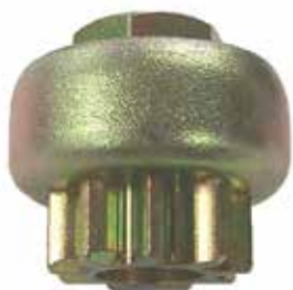
18-5650 STARTER DRIVE ASSEMBLY Replaces: Mercury/Mariner 57380
