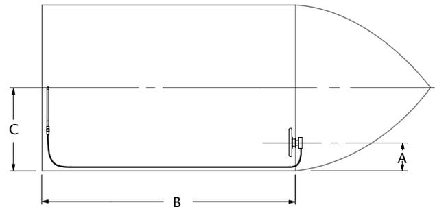
A single-cable, starboard drive push-pull mechanical cable system is shown in this diagram. If your mechanical system is different than the one depicted and/or you have any questions about mechanical steering after reviewing this guide, please contact SeaStar Solutions Technical Service.
