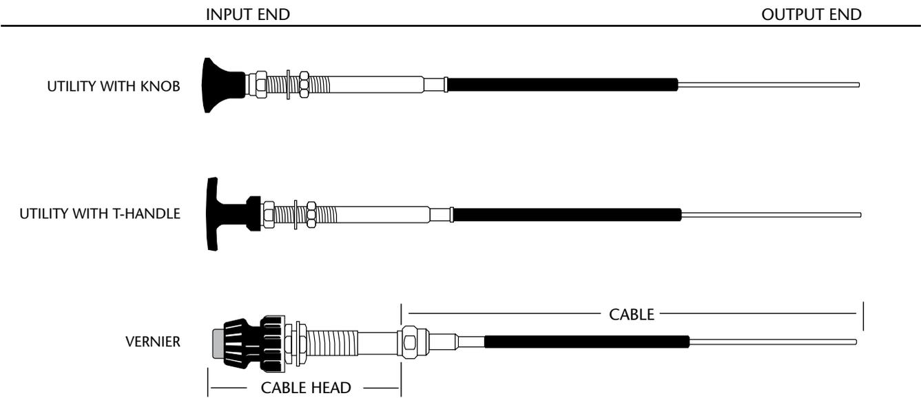
Note: The Marine Utility and Vernier control cable has a bare conduit at the output end with a .075 stainless steel wire.
