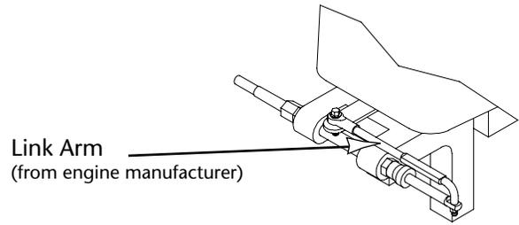
Parts Required: Engine Manufacturer's Link Arm
