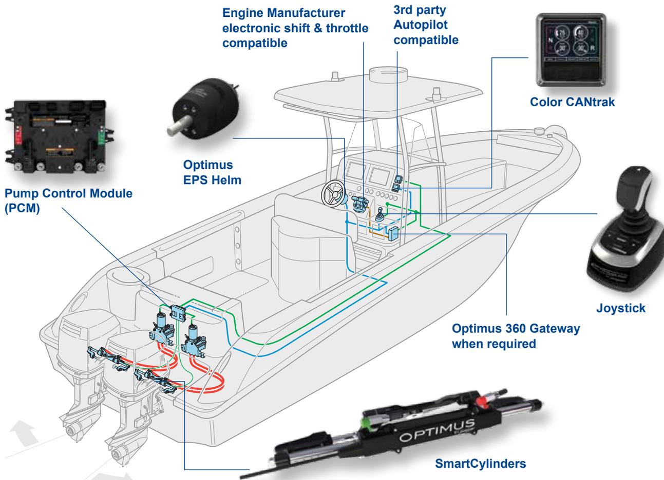
**Optimus EPS + Joystick = Optimus 360 Joystick Control**
