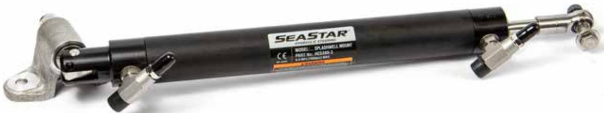
This cylinder is a light duty alternative to front & side mount cylinders. It is unbalanced with 5.5/6.5 turns lock-to-lock and fits engines with/without support (steering) tube. The splashwell mount cylinder is for single & multiple engine capability and has total power to 600 HP in counter rotating application. It can be transom or hull mounted cylinder. **NOTE: Not for use with SeaStar Pro helms.**
