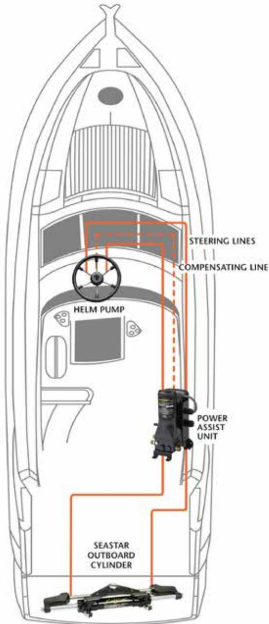
TYPICAL POWER ASSIST APPLICATION IN AN INBOARD BOAT
