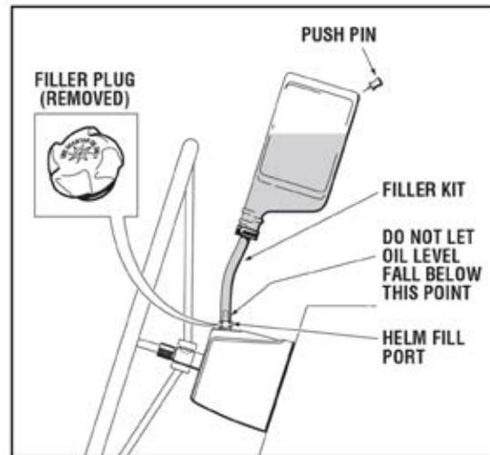
In an emergency, SeaStar EPS Fluid, any MD-3/4 rated ATF or MIL-PRF-5606H equivalent fluid that is filtered through a fine mesh screen can be used. The system MUST be thoroughly flushed as soon as possible with genuine SeaStar Steering Fluid after using an emergency fluid. In an EXTREME emergency, any non-toxic, non-flammable fluid that is filtered through a fine mesh screen may provide temporary steering.
