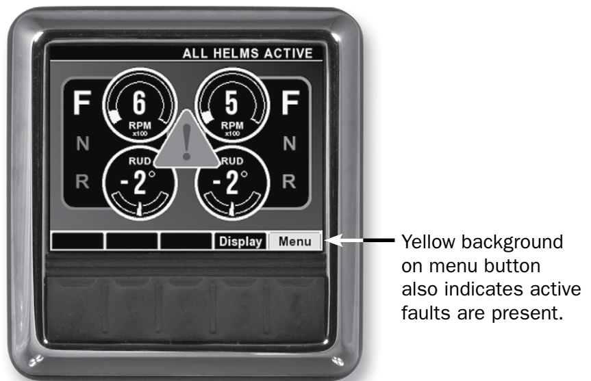
Figure 6-4. Run screen with system warning.
