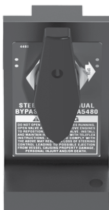
Figure 3-5 Remote steering service valve.
