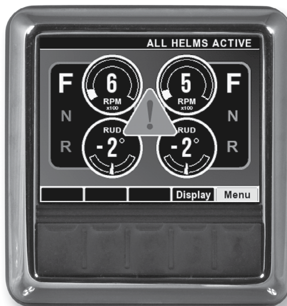
Figure 10-6. Run screen with system warning.
