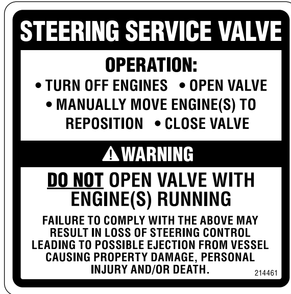
Figure 1-5. Steering service valve labels.
