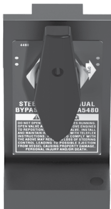
Figure 3-8 Remote steering service valve.
