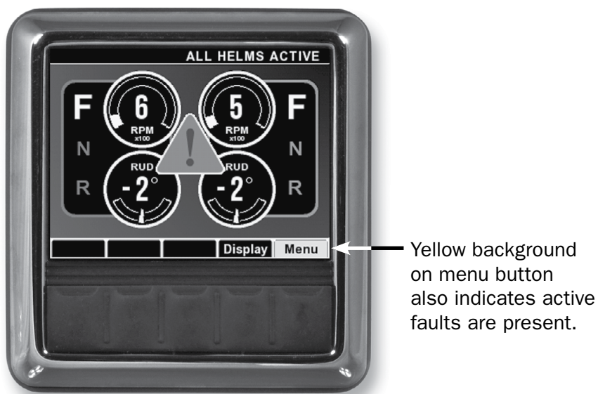
Figure 7-4. Run screen with system warning.
