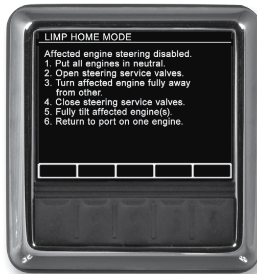
Figure 7-3. Limp home instructions, no steering on one engine.
