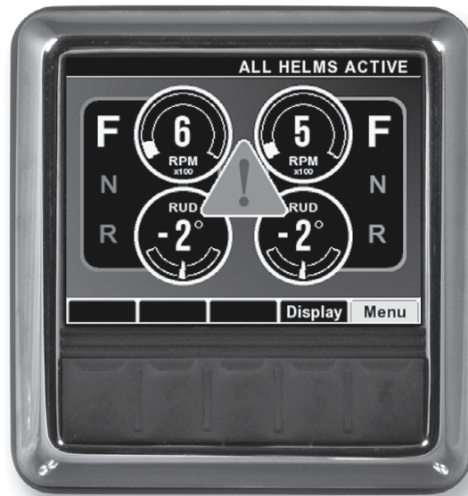
Figure 10-2. Run screen with system warning.
