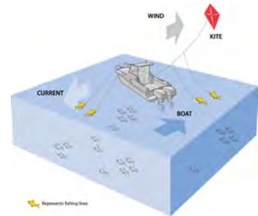
In the “heading hold” mode, SeaStation will hold the designated course heading. The boat holds its course heading, with the bow pointed in the heading direction, while allowing the vessel to drift with wind and/or current.
