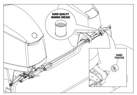
Figure 13. Cap Seal Installation.
