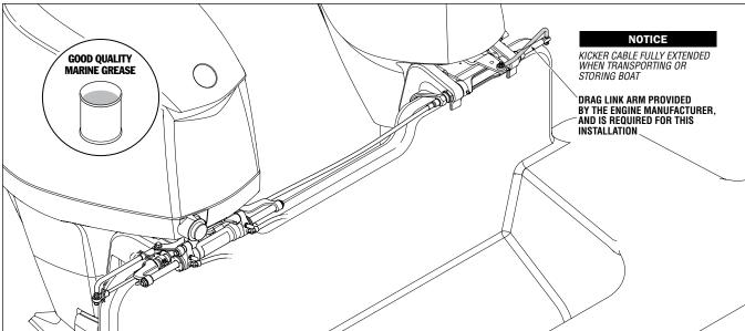
Figure 2. Additional parts required to complete installation.
