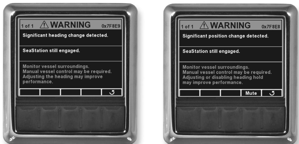
Figure 3-4. SeaStation Drift Faults.
