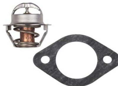
23-3659 THERMOSTAT KIT Temperature Rating: 140° Replaces: Westerbeke 37387 & 37922 Fits: 4.5 BCG(60Hz)/3.75 BCG(50Hz), 7.0 BCG(60Hz)/5.0 BCG(50Hz), 7.0 BCGA(60Hz)/5.0 BCGA(50Hz)
