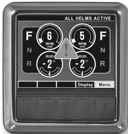
Figure 9-3. Run screen with system warning.
