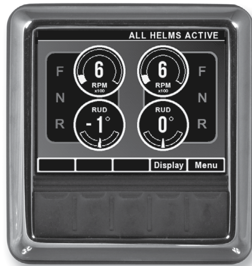
Figure 7-1. CANtrak display, All Helms Active screen.
