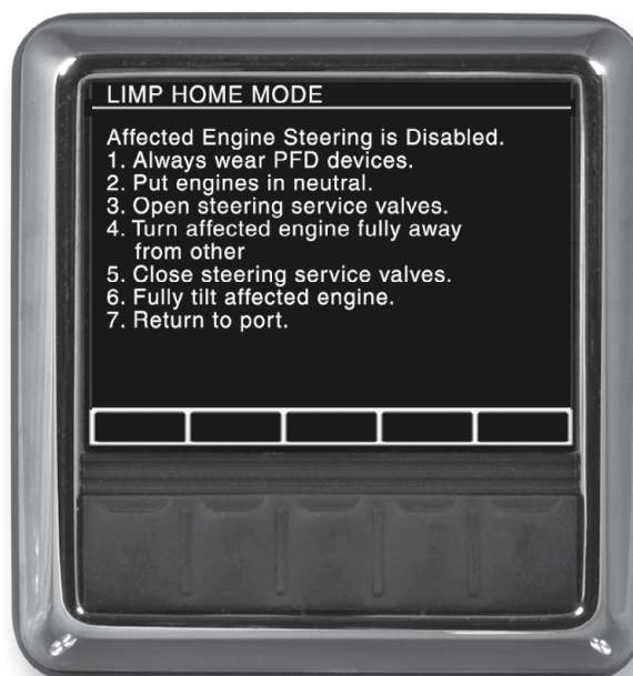
Figure 10-3. Limp home instructions, no steering on one engine.
