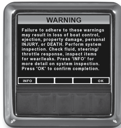
Figure 8-2. CANtrak initial warning screen.
