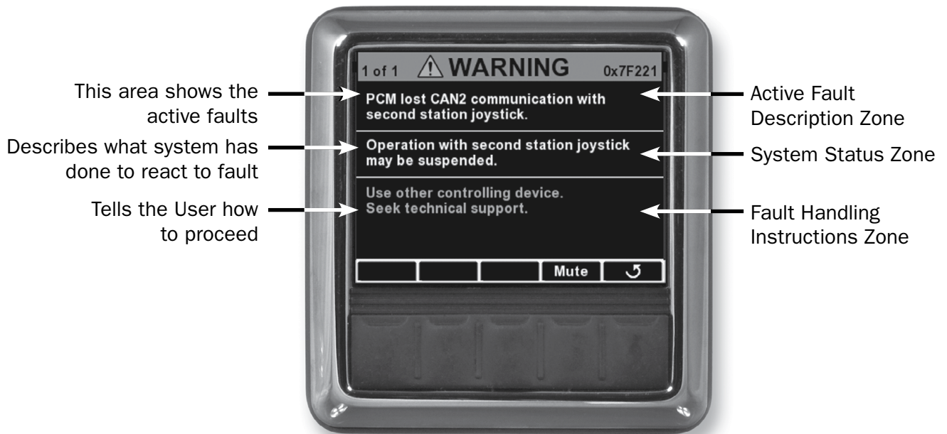
Figure 10-7. Sample warning fault.
