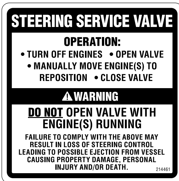
Figure 1-5. Steering service valve labels.
