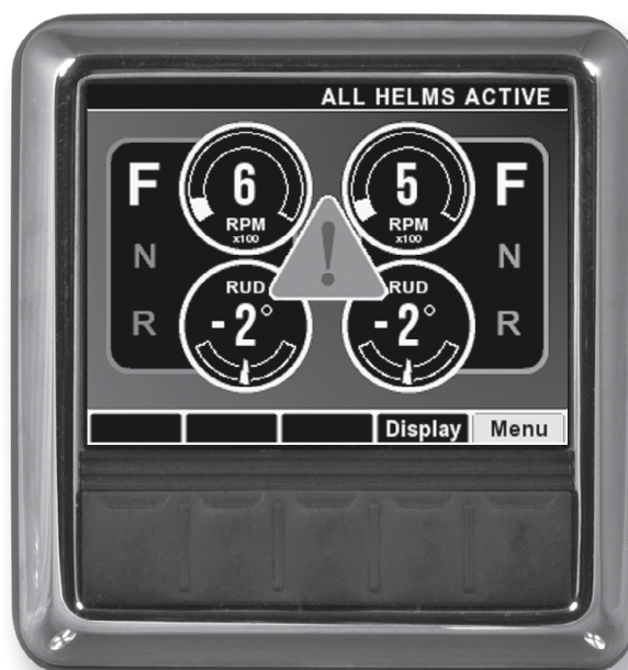
Figure 10-6. Run screen with system warning.
