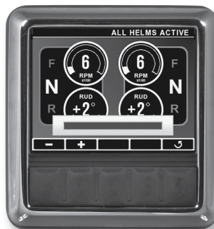
Figure 7-7. Display adjustment screen.
