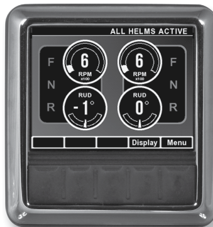
Figure 8-3. All Helms Active screen (normal steering mode).
