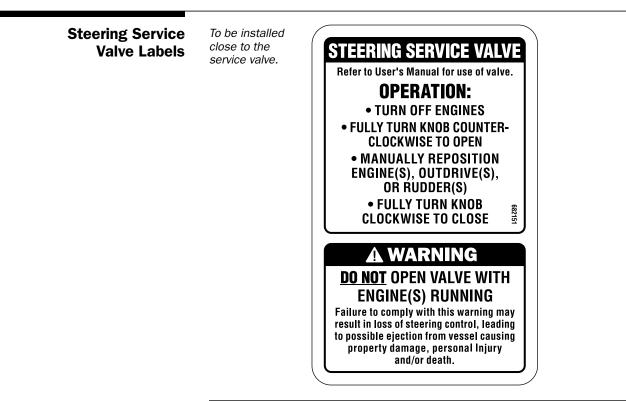
Figure 1-4. Steering service valve label.
