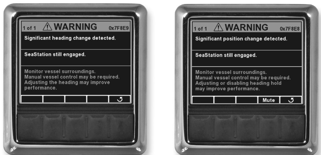
Figure 3-4. SeaStation Drift Faults.
