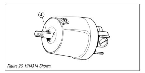
Remove steering wheel; clean off helm pump shaft; regrease using a good quality marine grease .
