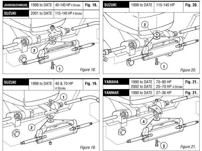
A WARNING In some cases, engine manufacturers will install plugs, caps and/or screws into the engine tiller arm. These plugs, caps and/or screws MUST be removed prior to installation of the steering cylinder. Failure to do so may cause wear on steering parts leading to property damage and/or personal injury or death.
