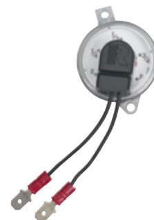
035760-10 Conversion Capsule Converts fuel level reading from standard direct site gauge to electric dash-mounted gauge (33-240 ohms).
