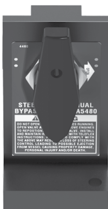
Figure 3-5 Remote steering service valve.
