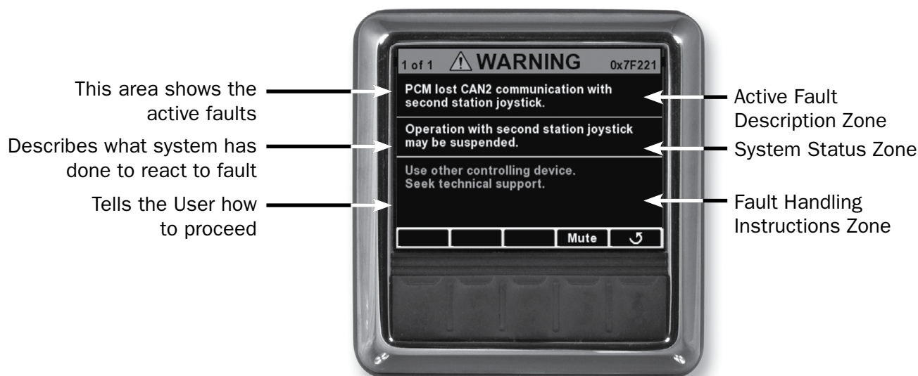
Figure 6-5. Sample warning fault.
