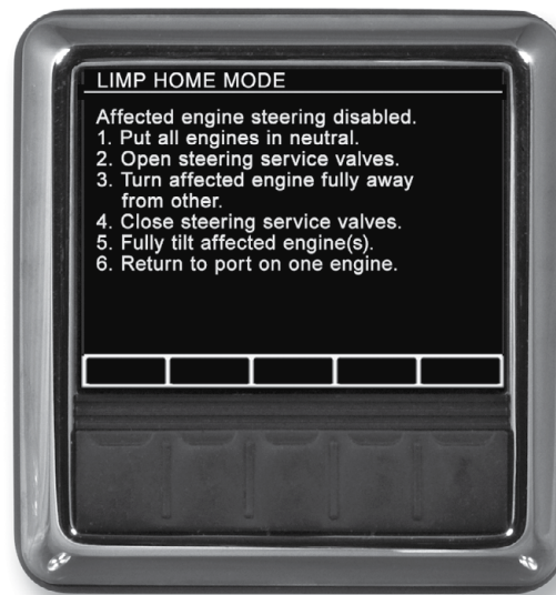
Figure 6-3. Limp home instructions, no steering on one engine.
