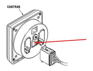
The USB connection access is located on the back of the CanTrak display.
